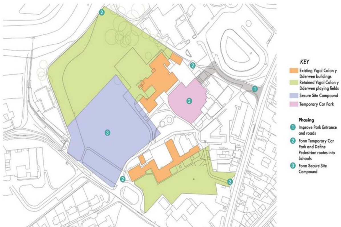
Figure 31: Construction sequencing and operation of the school
